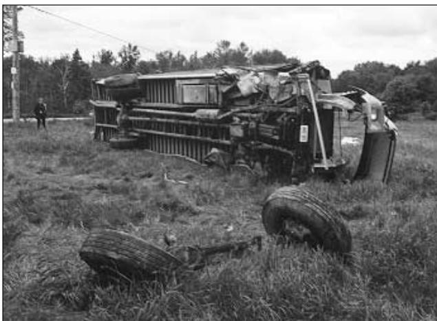
FIG. 1. Structural damage to front end and axle of bus in its final resting place.
