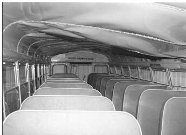
FIG. 2. The site of maximal roof intrusion lies toward the front of the bus cage.
