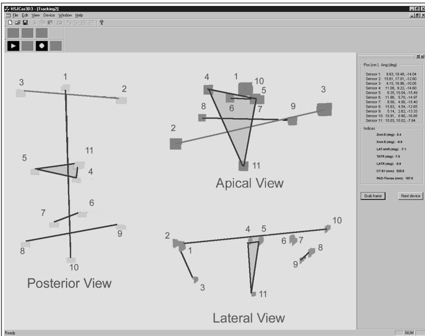
FIG. 4. Computer display of sensor positions, the geometric indices and the schematic representation of the trunk
