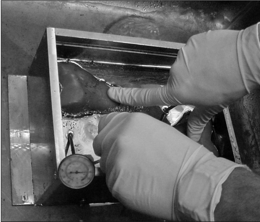
FIG. 1. Pair of distal femurs held in the aluminum frame containing 70°C Cerrobend (Cerro Metal Co.) with the anterior metaphysis exposed while cooling in a water bath to set the Cerrobend.
