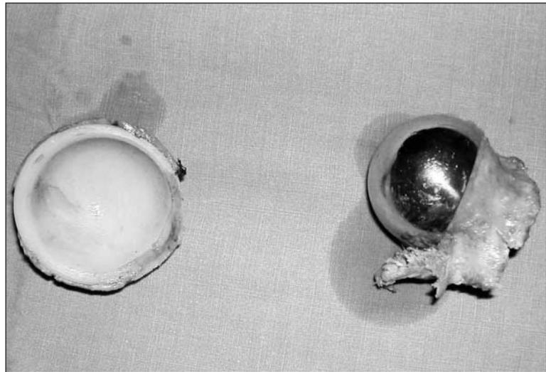
FIG 2. The resected components and femoral neck of the THARIES, 23 years after the resurfacing procedure.
