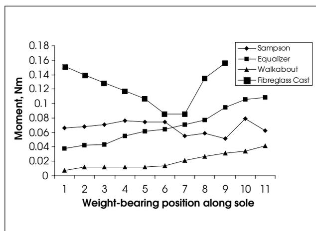
FIG. 4. Moment measurements (Nm) for each of the boots and the fibreglass cast at different positions (measurement 1 = heel, measurement 11 = toe), 2 cm apart, along the sole of the foot of cadaver foot 2.
