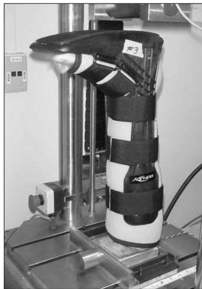
FIG. 2. A cast boot applied to the cadaver specimen and mounted in the test frame in readiness for the application of a force ranging from 0 to 70 kg over 7 seconds.
