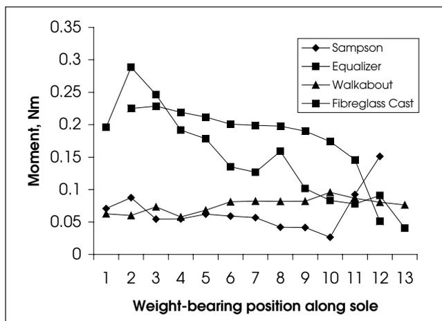
FIG. 3. Moment measurements (Nm) for each of the boots and the fibreglass cast at different positions (measurement 1 = heel, measurement 13 = toe), 2 cm apart, along the sole of the foot of cadaver foot 1.
