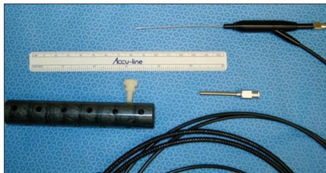
**Fig. 1.** Our first 4 FiberTech (0.7-mm external diameter) ductoscopes broke during the sterilization process at the junction of the metal scope and the plastic handle. Hospital engineers designed and built the perforated silicone sleeve (lower left), which fits over the scope when not in use to protect the junction and to allow for instrument sterilization. The metal cannula protects the junction when the surgeon uses the scope.
