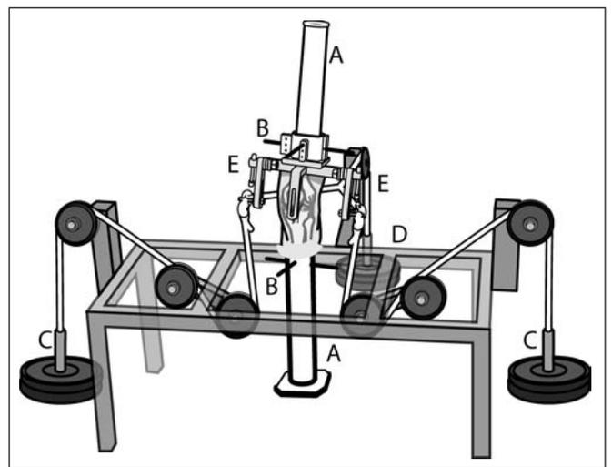
**Fig. 1.** Schematic showing the axial and anterior-posterior (AP) loading of intact knee specimens before and after anterior opening wedge high tibial osteotomy: (A) potted bone, (B) transfixion pins, (C) axial load application via weights, (D) AP load application via weights and (E) femoral markers. An overhead camera was used to track the motion of the femoral markers.
