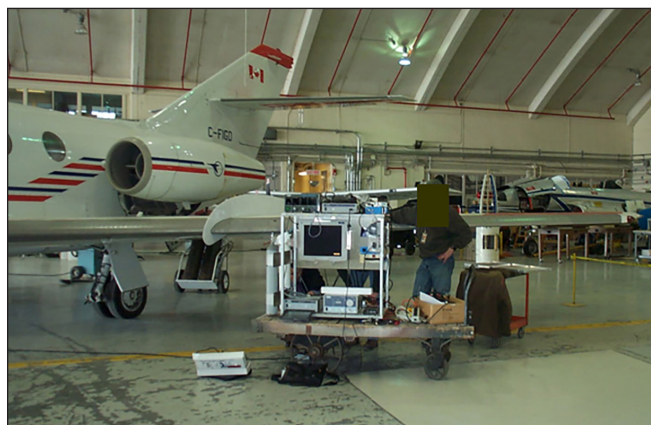
Fig. 6. Porcine life support and surgical work station before loading. An aeromobile modular critical care, resuscitation and surgical suite for operational medicine was developed to support surgery in variable gravity on-board the Falcon 20 Aircraft. Photograph taken by Andrew W. Kirkpatrick.
